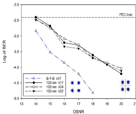
**Fig.3 *BER* curves for DL at B-t-B and 100 km span (Inset:  $\lambda_{17}$  corresponding constellation diagrams)**
