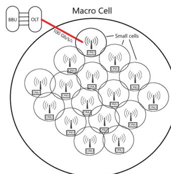
**Fig.1 The required bandwidth for 1 600 Gbit/s 5G MFH/MBH based PON technology**
