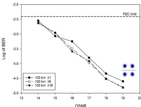
**Fig.4 *BER* curves for uplink at 100 km span of SMF (Inset:  $\lambda_{16}$  corresponding constellation diagram)**
