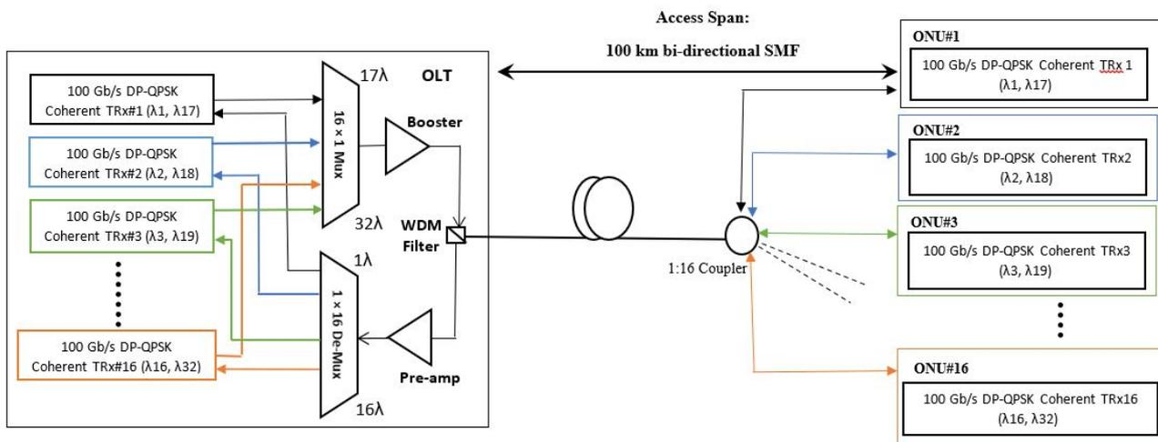
Fig.2 Architecture of the 1 600 Gbit/s coherent WDM PON system
