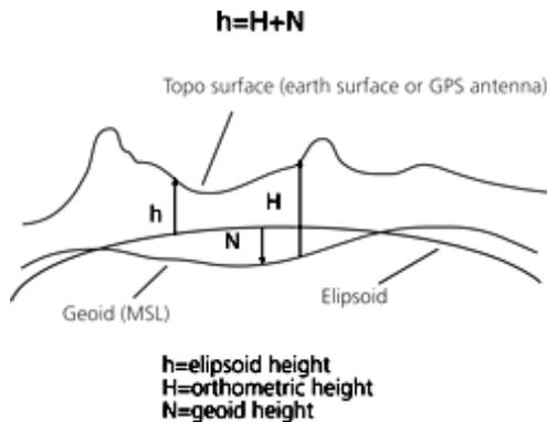
FIGURE 1: THE RELATIONSHIP BETWEEN THE DIFFERENT MODELS OF THE EARTH SURFACE
