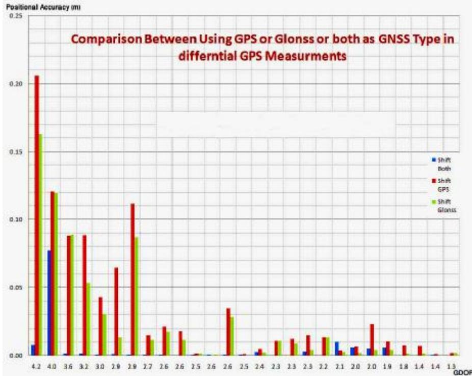
**Figure 3: Position variations and Geometric Dilution of Precision (GDOP) relationship.**
