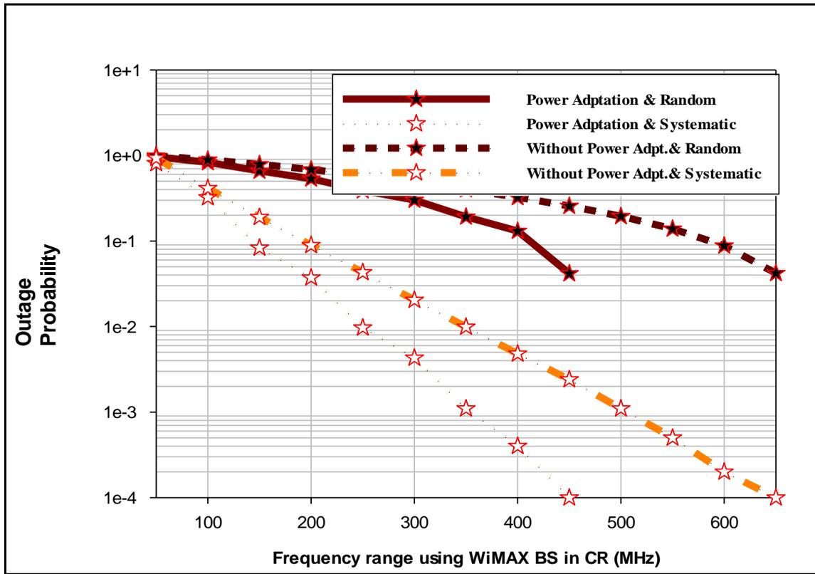
Figure 4.1: Outage probability of WiMAX CR application vs. TVWS frequency range.
