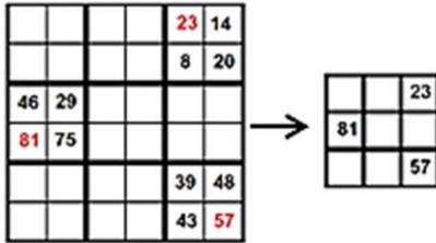
Figure 12. Max Pooling 2
