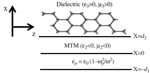
**Fig. 1.** The proposed structure. The field is assumed to travel a long the  $x$ -axis.
