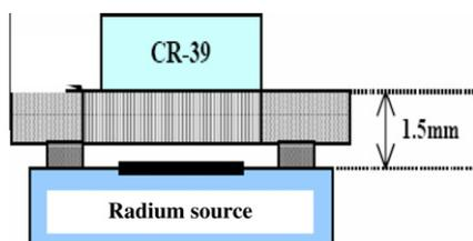
**Figure 1** Measurement technique for a solid radium source.
