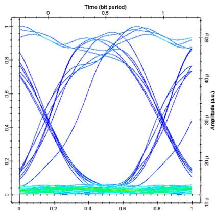
Fig. 3. Eye diagram of de-mod OOK signal-uplink.
