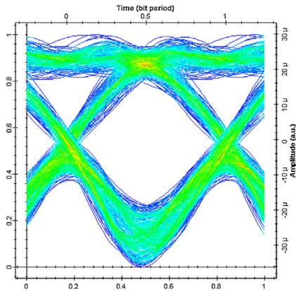
Fig. 2. Eye diagram of de-mod DPSK signal-downlink.
