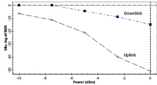
Fig. 4. BER versus input optical power.
