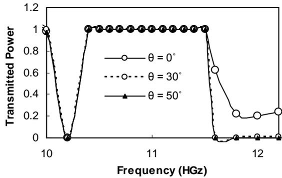
Figure 4. The transmitted power as a function of frequency when  $n_2 = |n_3|$ ,  $n_1 = n_4$  and  $a = d$  for various angles of incidence.
