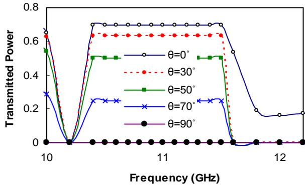
Figure 5. The transmitted power as a function of frequency when  $n_1 \neq n_4$ ,  $n_2 = |n_3|$  and  $a = d$  for various angles of incidence.
