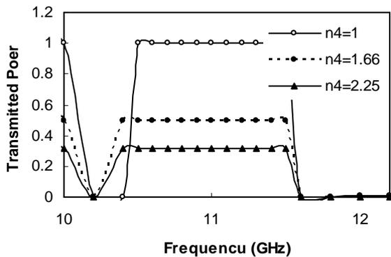
Figure 6. The transmitted power as a function of frequency when  $n_1 \neq n_4$ ,  $n_2 = |n_3|$ ,  $a = d$  and the angle of incidence  $\theta = 30^\circ$  (kept constant) for different values of  $n_4$ .
