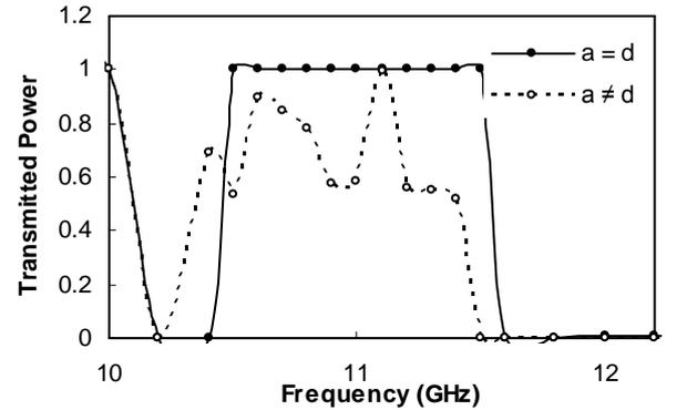
Figure 3. Transmitted power variation with frequency when  $n_1 = n_4$ ,  $n_2 = |n_3|$  and  $\theta$  kept constant for two cases with respect to the widths  $a$  and  $d$  of the slabs: (a)  $a=b$ ; (b)  $a \neq d$ .
