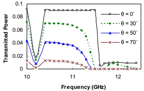
Figure 7. The transmitted power as a function of frequency where the condition ( $n_1 < n_2$ ,  $n_2 > n_3$ ,  $n_3 < n_4$ ) is satisfied for various angles of incidence.
