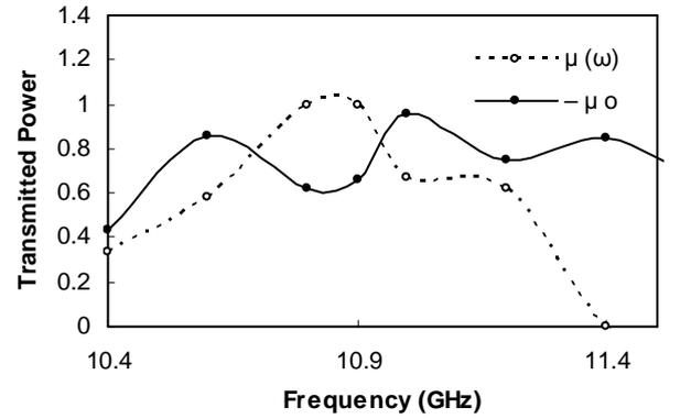
Figure2. Transmitted power variation with frequency. Two cases are taken into account: (a)  $\mu_3$  is a function of  $\omega$ ; (b)  $\mu_3$  is a constant ( $-\mu_0$ ).
