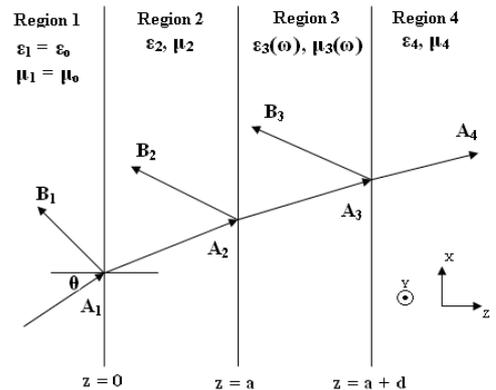
Figure 1. Wave propagation through a structure consisting of a pair of dielectric and metamaterial embedded between two dielectric semi-infinite media.
