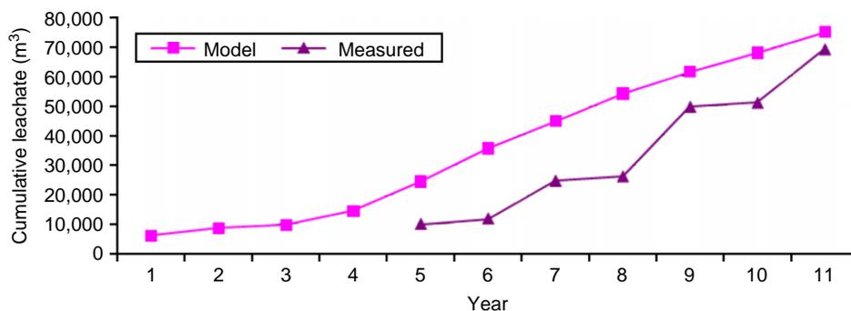
**Figure 5** | Measured and estimated cumulative annual leachate volume generated at Dear Al Balah landfill.
