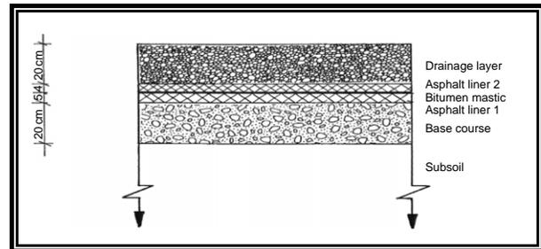
Figure 4 | Asphalt lining system cross section at Dear Al Balah landfill (GTZ 1996).
