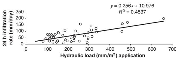
Fig. 4. Twenty-four hour infiltration rate versus hydraulic load (planted bed).
