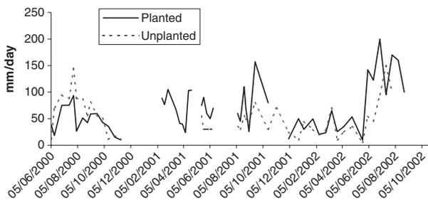
Fig. 3. Twenty-four hour infiltration rate (mm/day).
