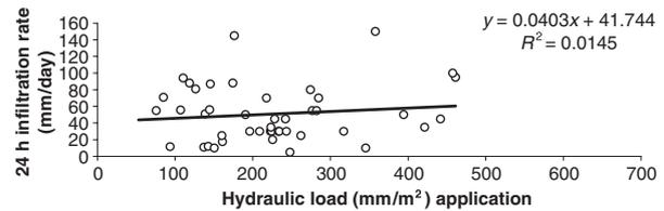
Fig. 5. Twenty-four hour infiltration rate versus hydraulic load (unplanted bed).
