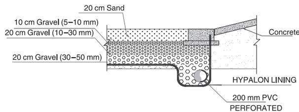
Fig. 1. Schematic diagram of reed bed cross section.
