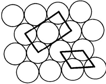
FIG. 1. Hexagonal parent model structure shown in plan with hexagonal and monoclinic unit cells.
