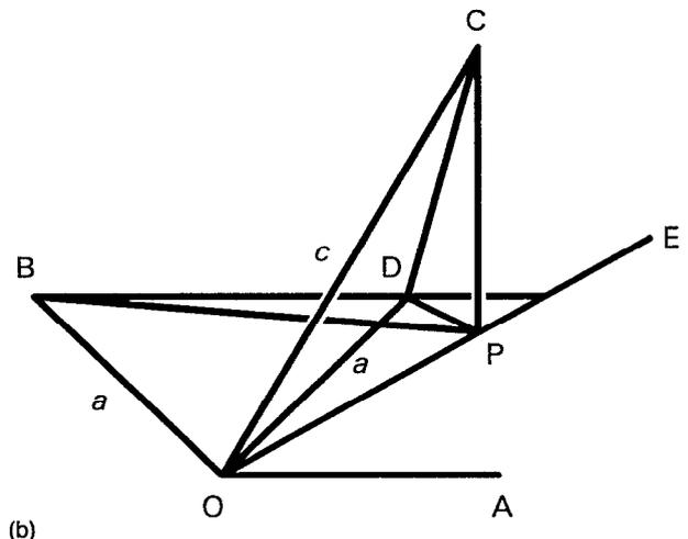
FIG. 3. Unit cell edges and construction for calculating unit cell angles in tilted structures (a) nearest-neighbor (NN) tilt; (b) next-nearest-neighbor (NNN) tilt.
