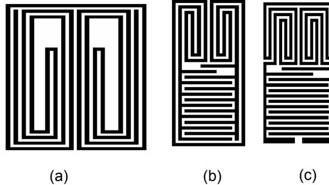
Fig. 1. (a) Dual spiral-in-spiral-out resonator; (b) Dual spiral-in-spiral-out resonator with capacitive load; (c) Modified capacitive-loaded spiral-in-spiral-out resonator.
