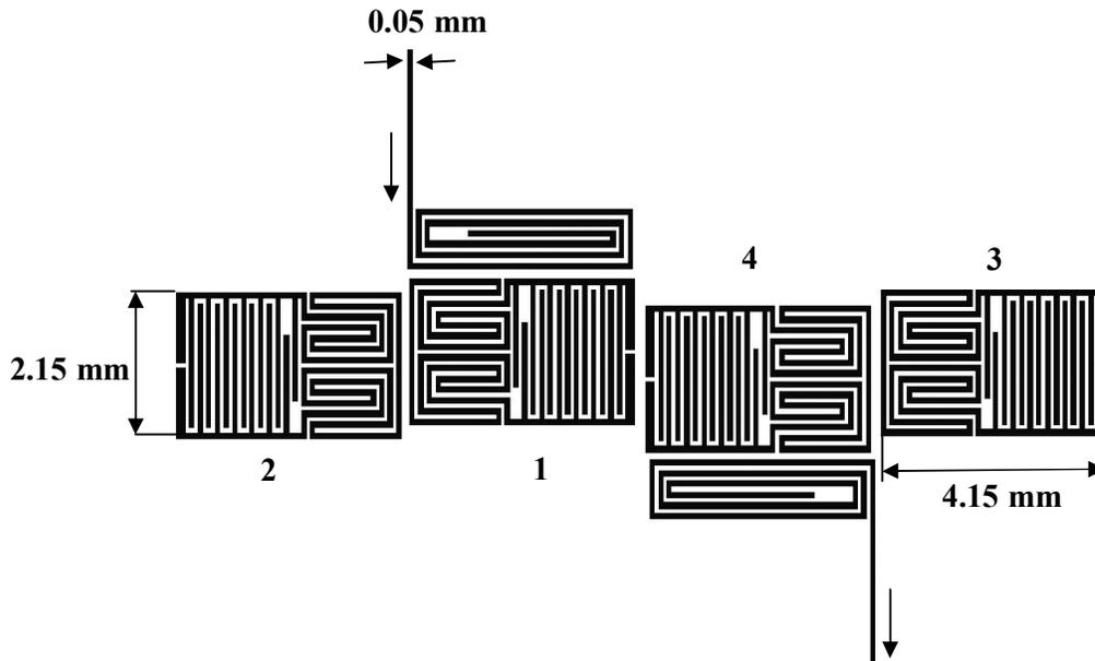
Fig. 3. Four-pole dual band filter layout.
