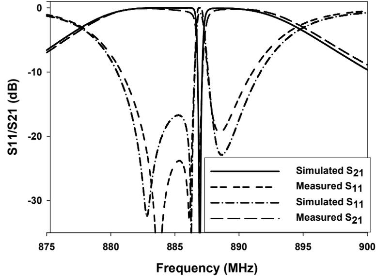
Fig. 4. Measured insertion and reflection losses of the 4-pole dual-band filter and the simulated responses.
