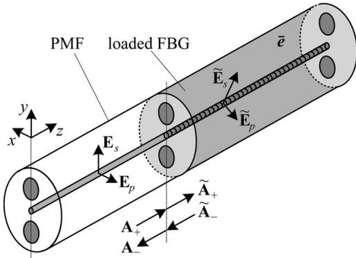
Fig. 1. FBG subject to a mechanical load ( $\bar{e}$ ). The fundamental modes of the FBG change their polarization due to the mechanical perturbation  $\bar{\underline{B}}$ .
