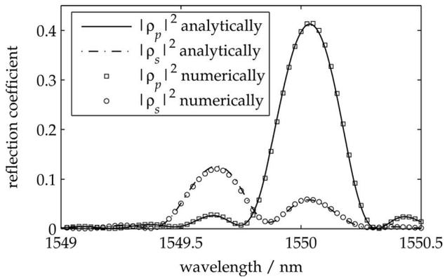
Fig. 2. Results for a grating with  $L_B=3.5$  mm,  $e_{xy}=1 \times 10^{-3}$ ,  $L=3$  mm, and  $\Delta n=1 \times 10^{-4}$ .
