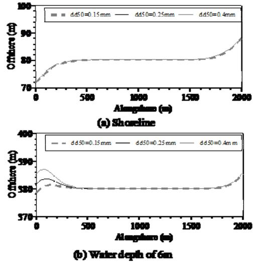
Figure 8. Difference of the nourished sand of the grain size for Case 2
