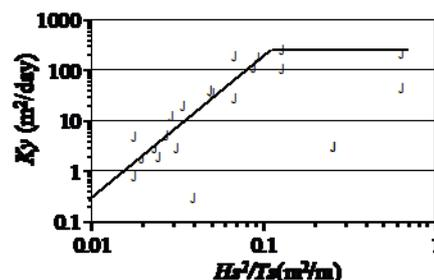
Figure 2(b). Diffusion coefficient in the longshore direction
