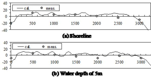
Figure 11. Comparison of the volume of contour line changes during 5 years
