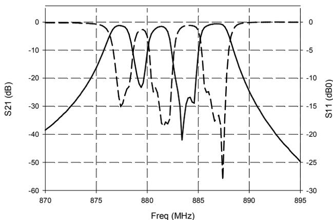
Fig. 4. Measured response of 10-pole triple-band HTS filter
