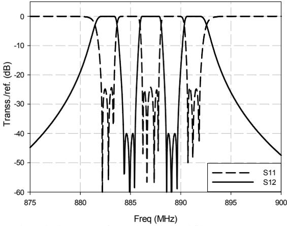
Fig. 2. Theoretical response of 10-pole triple-band filter
