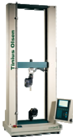
Figure 1: The Tinius Olson H10K materials testing machine
