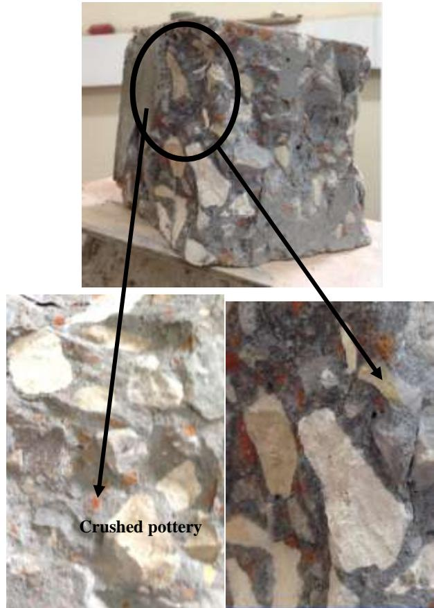
Figure 2. Well distribution of Crushed pottery particles
