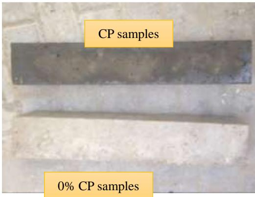
Figure 3. Wet appearance on the CP samples compared with 0% CP samples at 3 days age and room temperature.
