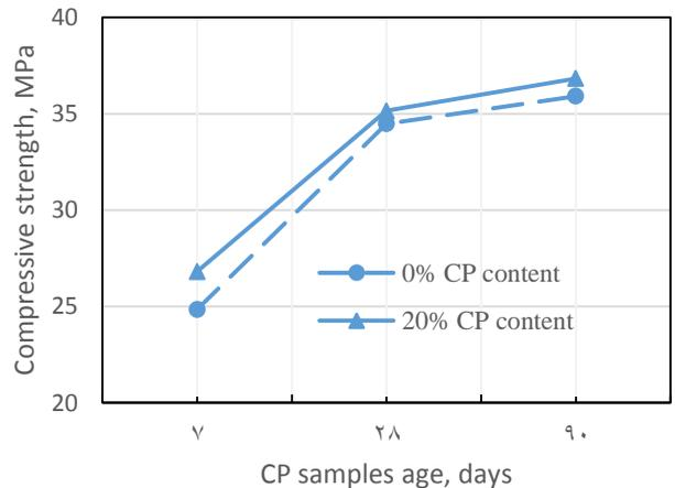
Figure 8. Compressive strength of 0% and 20% CP samples at 7, 28 and 90 days
