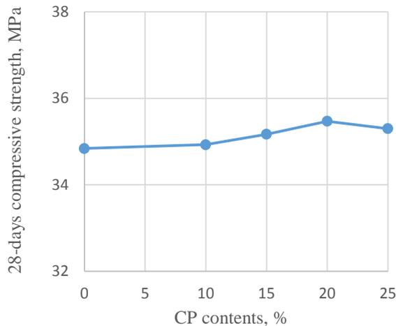
Figure 7. Compressive strength for CP samples at 28 days
