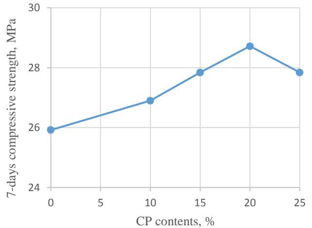
Figure 5. Compressive strength for CP samples at 7- days
