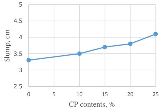
Figure 4. Slump values for CP samples
