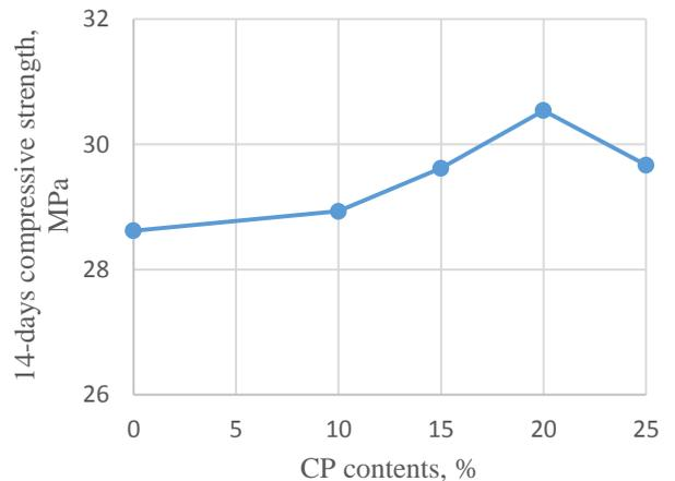
Figure 6. Compressive strength for CP samples at 14 days
