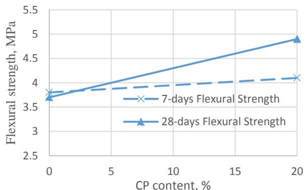
Figure 9. Flexural strength of 0% and 20% CP samples at 7 and 28 days.
