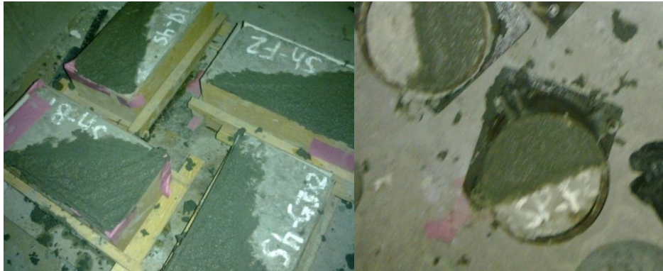
Figure 4: Slant shear and splitting test specimens.
