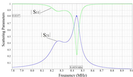
Figure 6. Simulated S-parameters for two-coil transmitter configuration.
