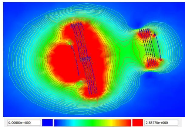
Figure 7. Magnetic field plots for two-coil transmitter configuration
