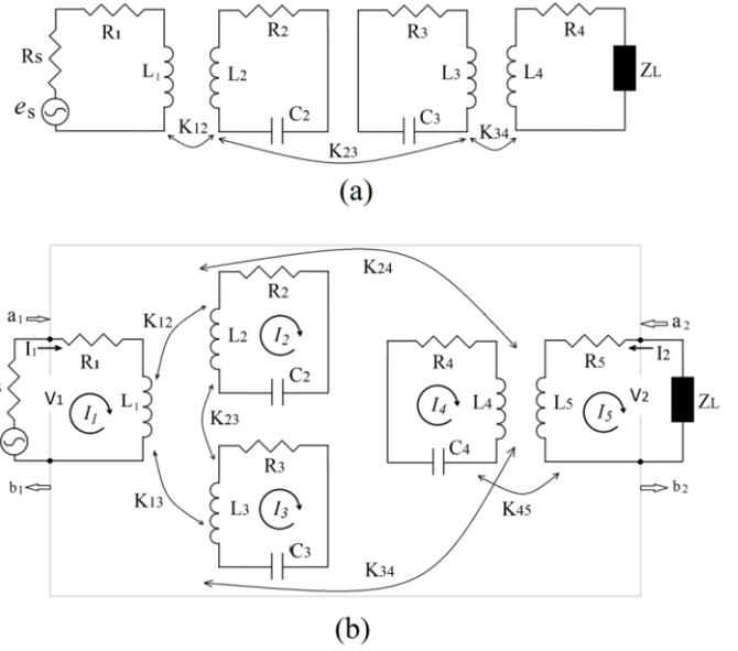
**Figure 2.** Equivalent circuit models for configurations in Figure 1 (a) Model for system in Figure 1 (a), (b) Model for system in Figure 1 (b).
