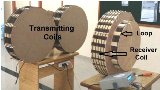
**Figure 8.** Experimental model for two-coil transmitter configuration
