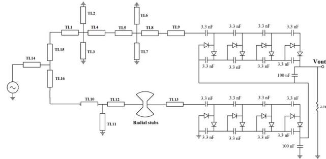
Fig. 4. Circuit diagram of the whole matching and rectifier system.
