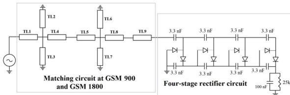
Fig. 2. Circuit diagram of the rectifier and matching circuit at GSM-900 and GSM-1800.
