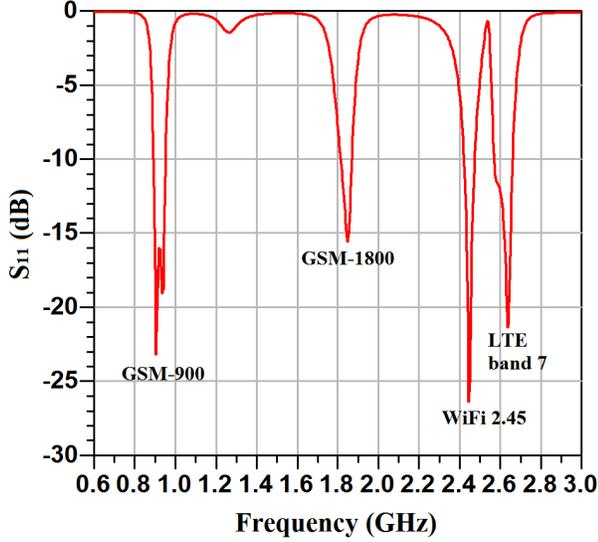
Fig. 11: Simulation result of  $S_{11}$  for circuit in Fig. 4.
