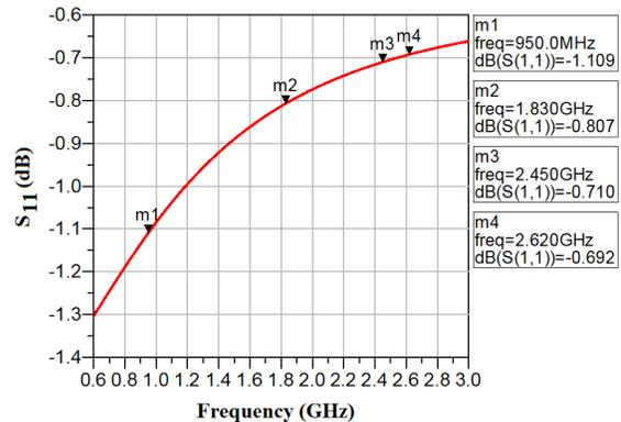
Fig. 6. Simulated  $S_{11}$  response of rectifier (without matching circuit).
