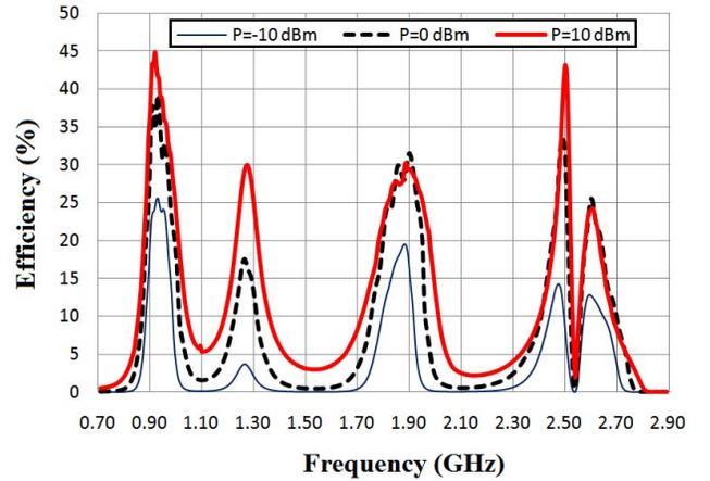
Fig. 13: Efficiency versus frequency for different input power levels with output voltage on 25 k $\Omega$ .
