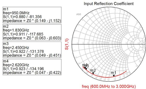
Fig. 5. Smith chart simulation results of rectifier circuit
