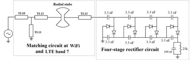
Fig. 3. Circuit diagram of the rectifier and matching circuit at WiFi and LTE band 7.
