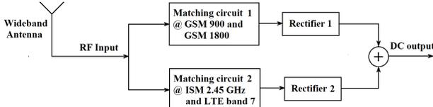
Fig. 1. Block diagram of the proposed quad-band harvesting system.
