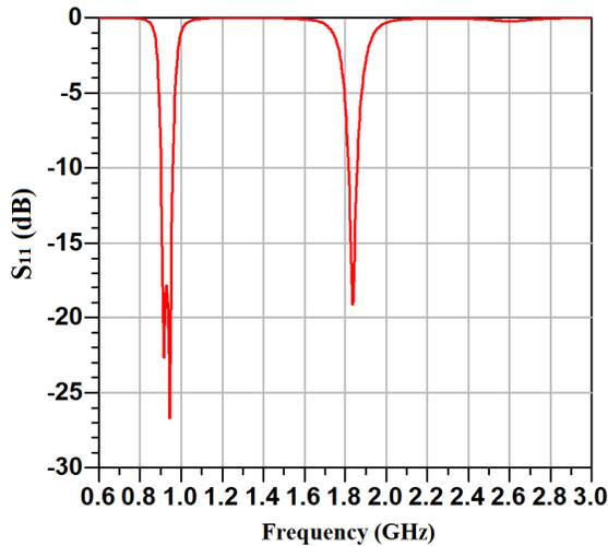
Fig. 7: Simulation result of  $S_{11}$  for circuit in Fig. 2.
