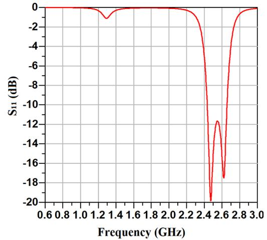
Fig. 9: Simulation result of  $S_{11}$  for circuit in Fig. 3.
