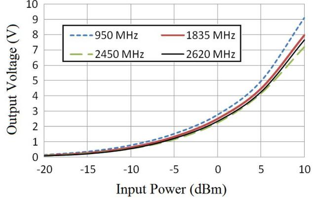
Fig. 12: Output DC voltage on 25 k $\Omega$  versus input power levels
