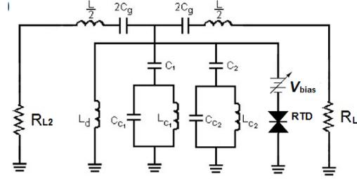
Fig. 2: VCO Equivalent circuit consists of the CLRTL unit cell loaded with RTD (Fig. 1) surrounded by two  $50 \Omega$  load resistances at the
