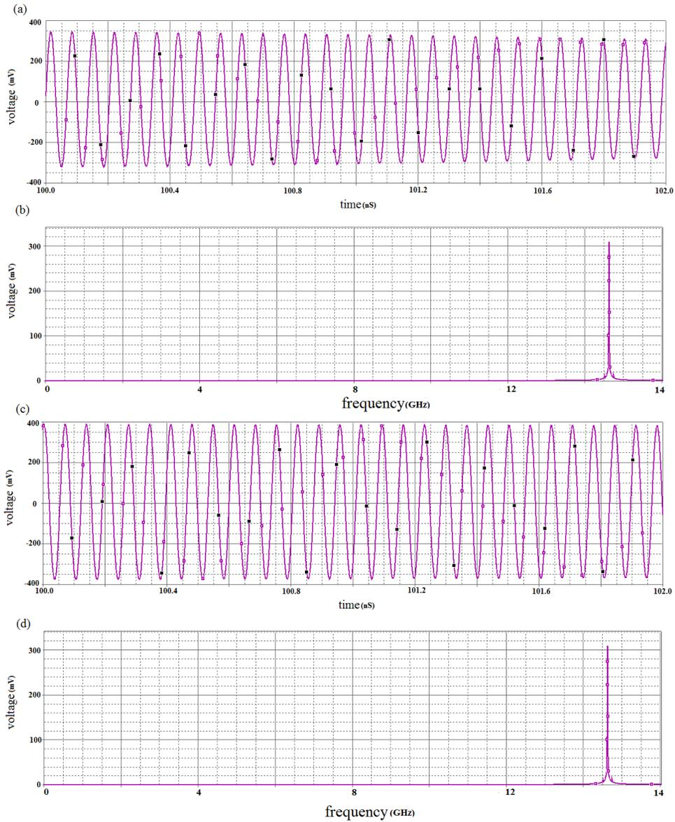
Fig. 3: The output voltage of our simulation measured in time domain and in frequency domain at two different values of  $V_{bias}$ . (a, b)  $V_{bias}$  equals 0.9V (c, d)  $V_{bias}$  equals 1.1V.
