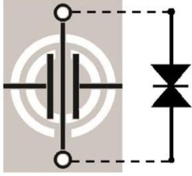
Fig. 1: RTD at shunt with grounded stubs of the hybrid CRLMTL cell.
