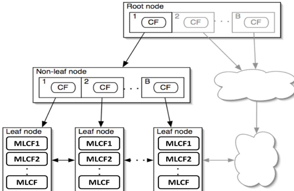
Figure 2. The Structure of Modified CF Tree
