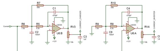
Figure 11. Current signal conditioning
