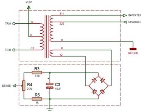
Figure 5. Feedback using additional winding
