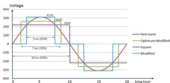
Figure1: Types of inverter output waveforms
