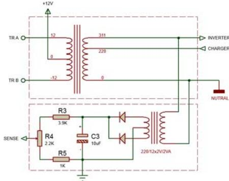
Figure 4. The power transformer and the feedback
