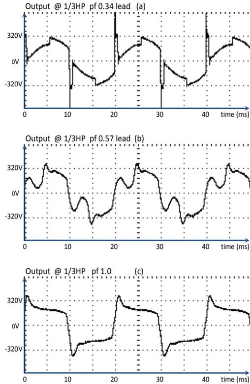
Figure 14: Output waveforms with a Fridge motor at different levels of power factor.
