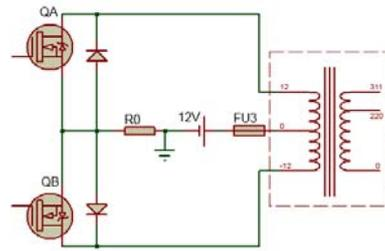
Figure 15. Additional freewheeling diodes
