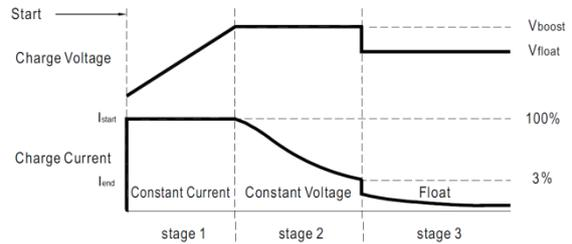
Figure 6. Three stage charging algorithm
