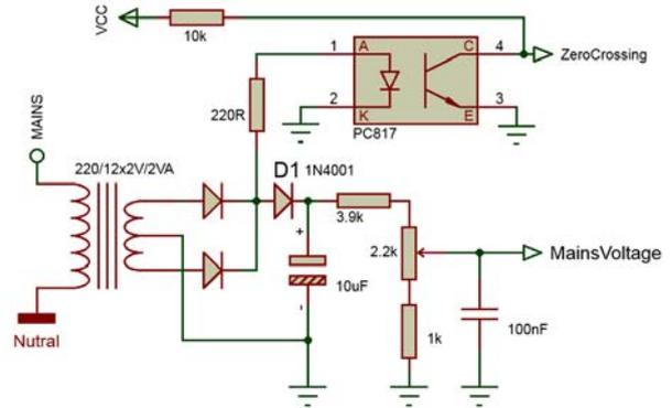
Figure 10. Modified AC mains sensing
