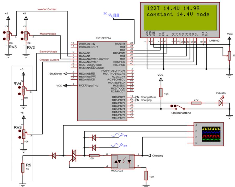
Figure 17. Charging algorithm simulation circuit.
