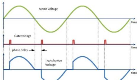
Figure 9. Phase angle control
