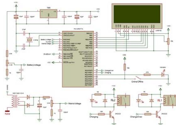
Figure 3. Device controller
