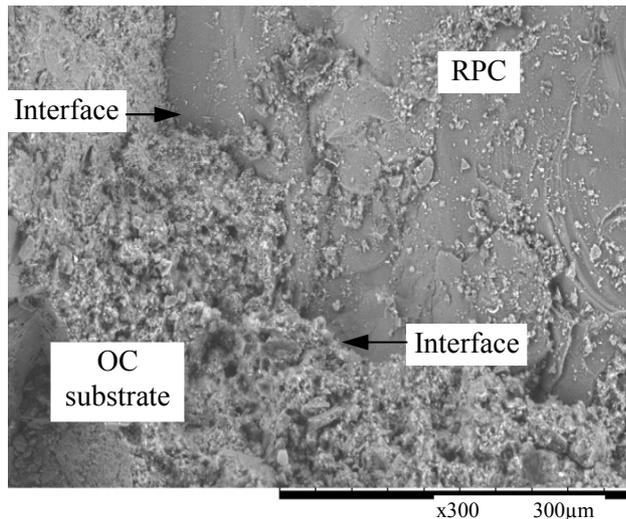
Fig. 3. SEM micrograph of the transition zone between OC substrate and RPC
