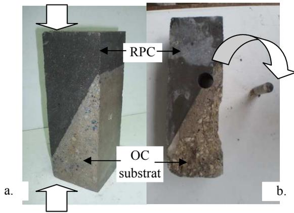
Fig. 1. a. Slant shear test specimens. b. Core sample extracted from the interface between OC substrate and RPC for SEM/EDX test
