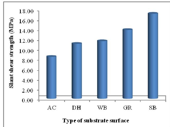
Fig. 2. Slant shear strength for each type of substrate surface
