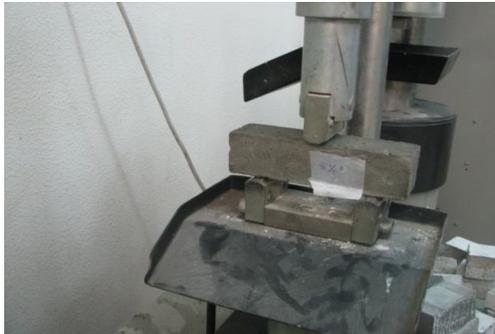
Figure 1.9 concrete cube during flexural test
