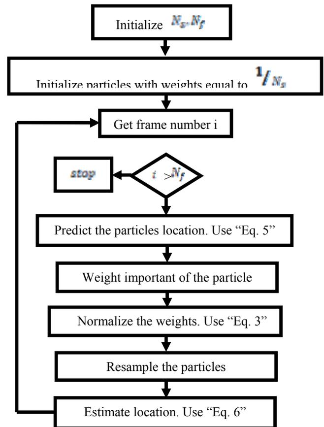
**Fig 1:** flow chart of video object tracking using PF
