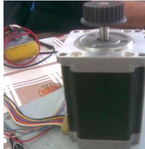
Figure (14): Unipolar Stepper Motor.
