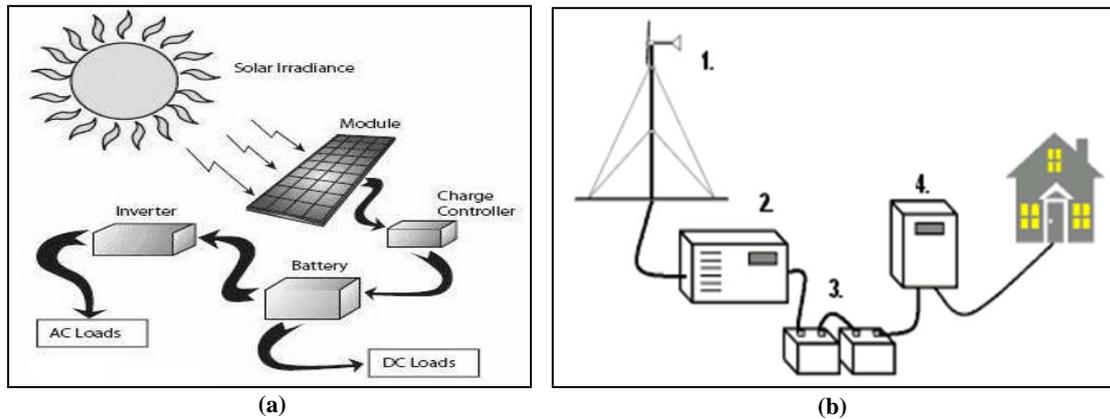
Figure (7): Stand- Alone Solar and Wind Energy Systems
