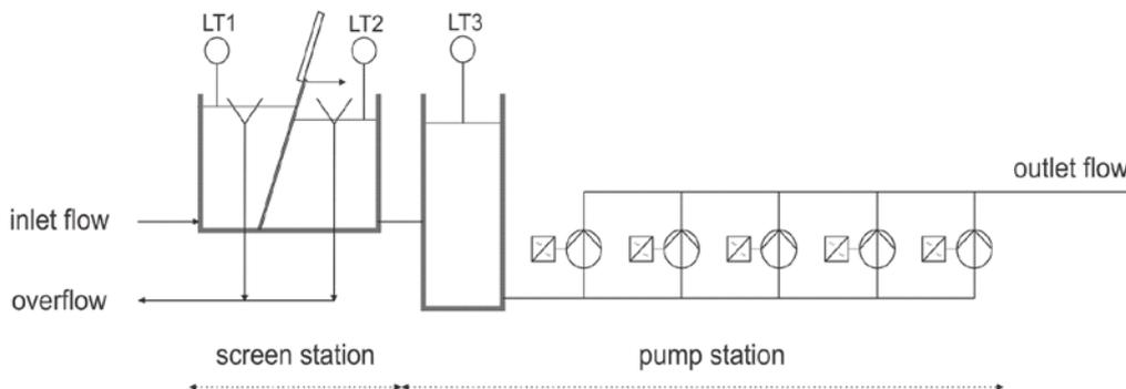
Figure 1: Process flow diagram of a typical wastewater pumping station
