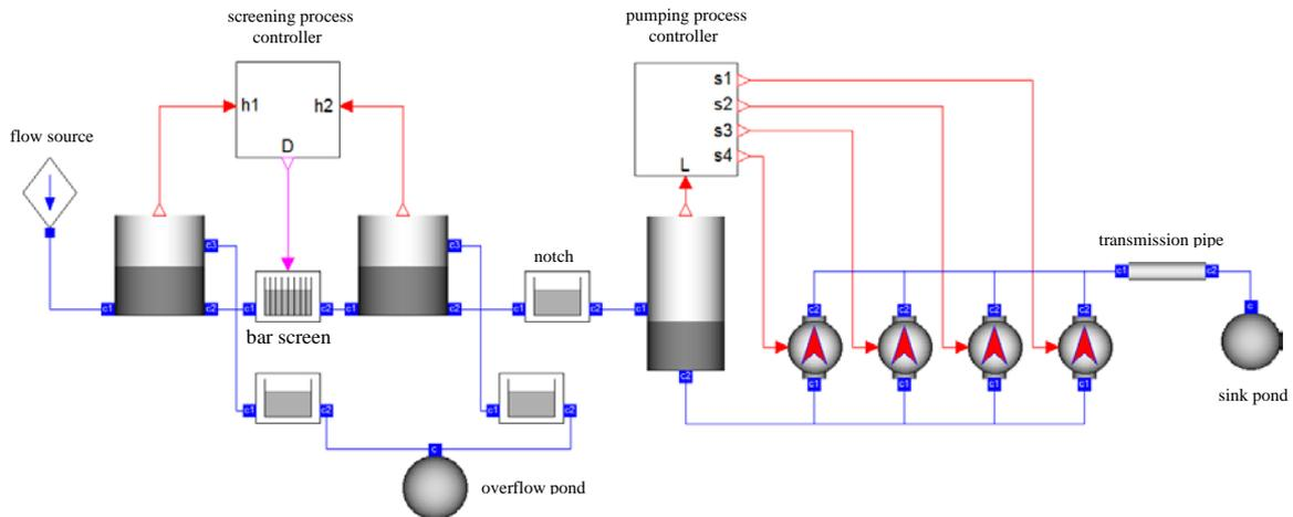
Figure 4: The top level model of the NTPS.
