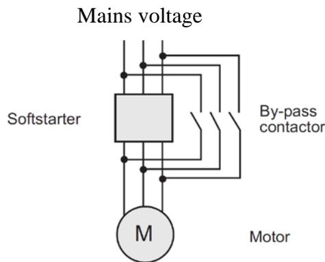
Figure 3. Bypass contactor use to minimize losses.
