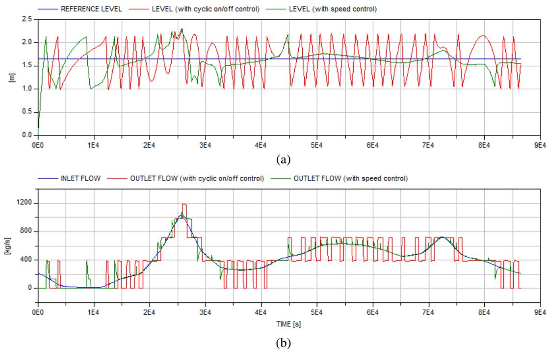
Figure 7. Level and flow variation under soft starters-based and frequency converters-based controllers
