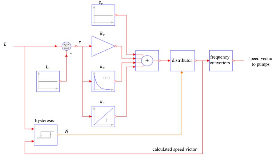
Figure 6. Block diagram of the PID-based variable speed controller
