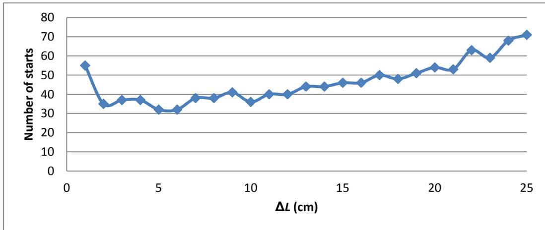
Figure 5. Variation of number of starts of pumps with respect to  $\Delta L$
