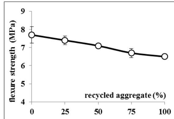
**Figure 6** Flexure strength of samples prepared by replacing aggregate less than  $360\mu\text{m}$  avec Super-plasticizer
