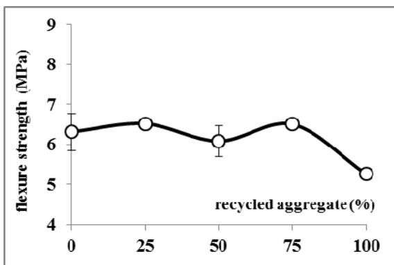
**Figure 2** Flexure strength of samples prepared by replacing aggregate less than 630µm
