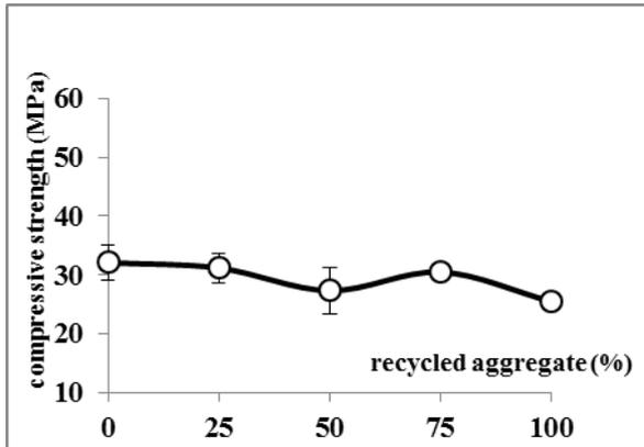
**Figure 1** Compressive strength of samples prepared by replacing aggregate less than 630µm
