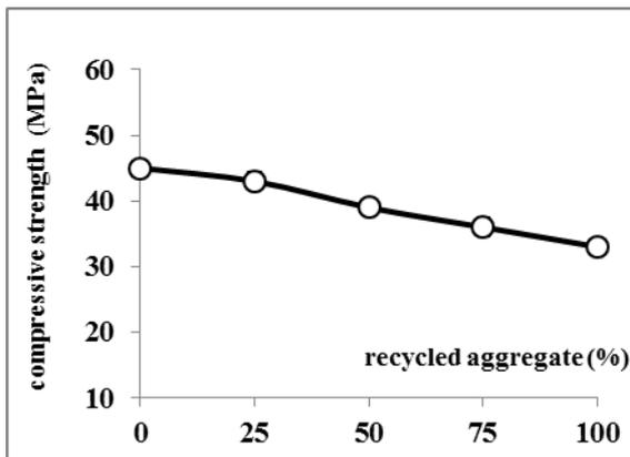
**Figure 5** Compressive strength of samples prepared by replacing aggregate less than  $360\mu\text{m}$  avec Super-plasticizer
