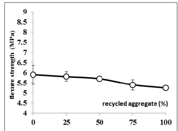
**Figure 4** Flexure strength of samples prepared by replacing aggregate less than 360µm
