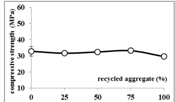
**Figure 3** Compressive strength of samples prepared by replacing aggregate less than 360µm
