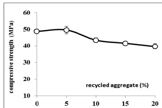
**Figure 7** Compressive strength of samples prepared by replacing cement by very fine RA
