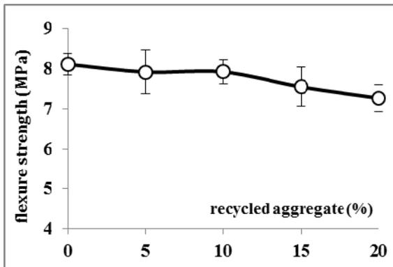
**Figure 8** Flexure strength of samples prepared by replacing cement by very fine RA
