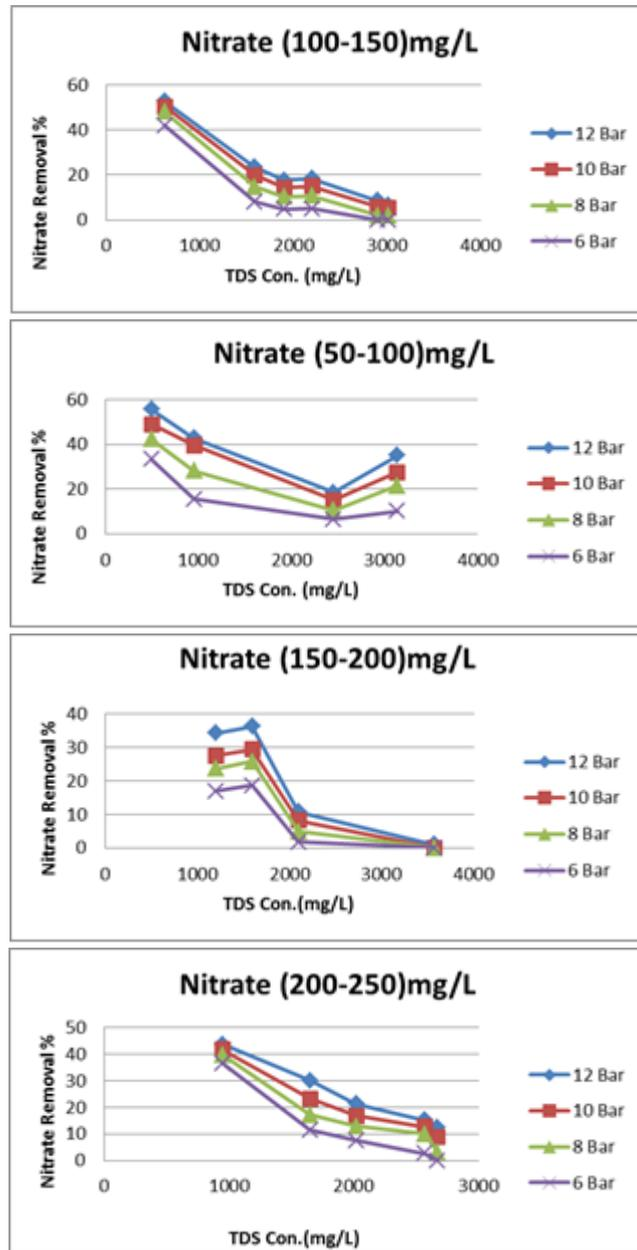
**Figure 7** Relation between TDS concentration and nitrate rejection
