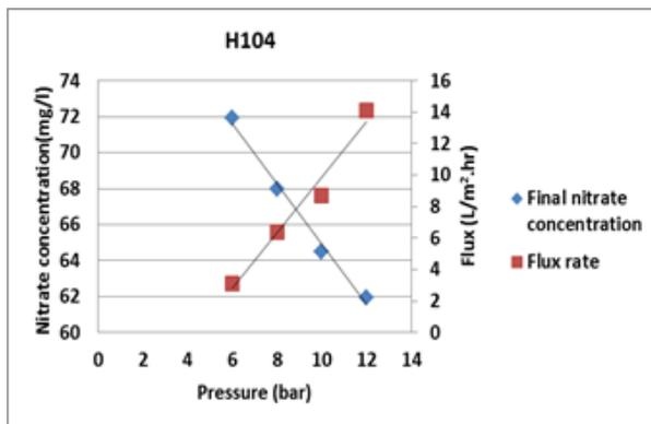
**Figure 9** H104 operation diagram
