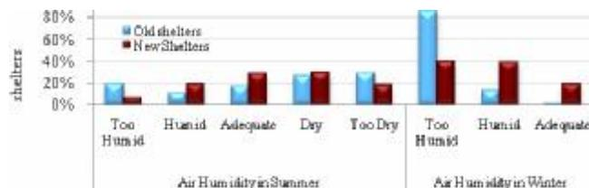
Figure 11: air humidity in old & new shelters
