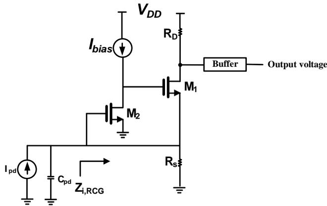
Fig. 2. Regulated common gate (RCG) TIA.
