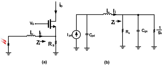
Fig. 3. The input part of a narrowband RCG TIA.
