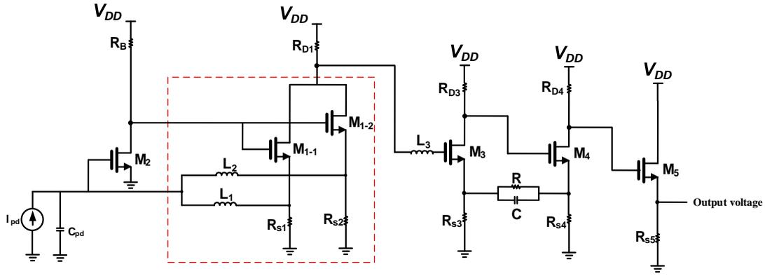
Fig.7. Schematic of proposed RCG TIA.
