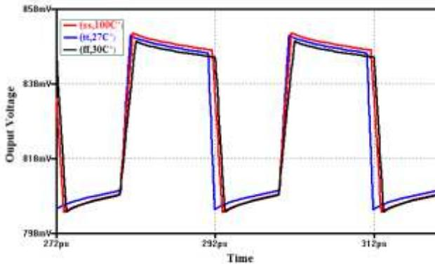
Fig.13. Transient response of the TIA at different process corners.
