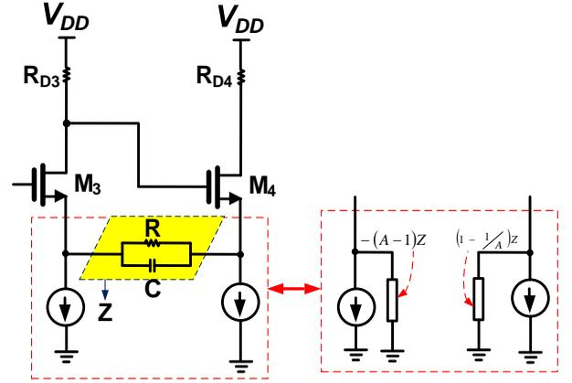
Fig.6. The proposed configuration of capacitive degeneration.
