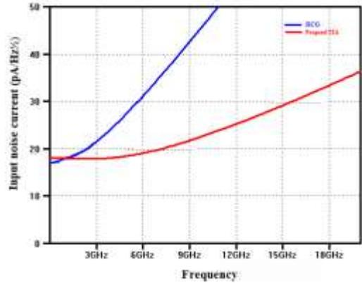
Fig.11. Spectral density of the input noise current
