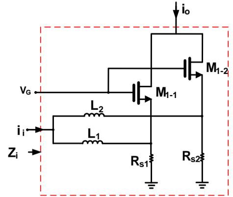
Fig. 4. The input part of RCG TIA with two input branches.
