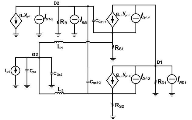
Fig.8. Modified RCG TIA with noise sources.
