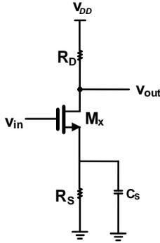
Fig.5. Configuration of capacitive degeneration.
