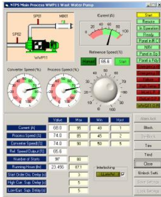
Figure 7. A wastewater pump display.
