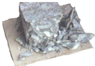
Figure 10: (a) Photograph of a concrete specimen showing significant surface cracking and spalling, indicating structural damage. (b) Microscopic view of a concrete surface showing yellow crystalline deposits. A red circle highlights a specific area of interest.
