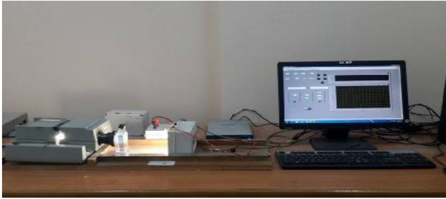
**Fig. 3.6** System of I-V measurement and solar cell simulator
